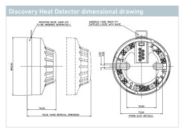
Note: Should be used with Deckhead Mounting Box - Part No. 45681-217 if ingress protection is required.
